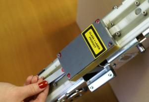
Attention: While insertion the cleaning pad has to face upwards!
